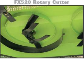
Close up of fixed knife technology with stationary mounted fixed knife and rear mounted baffle
